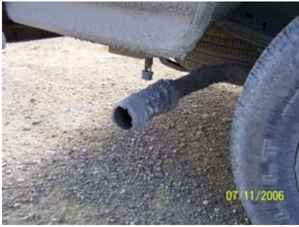
060711-38 mud accumulation on exhaust pipe
